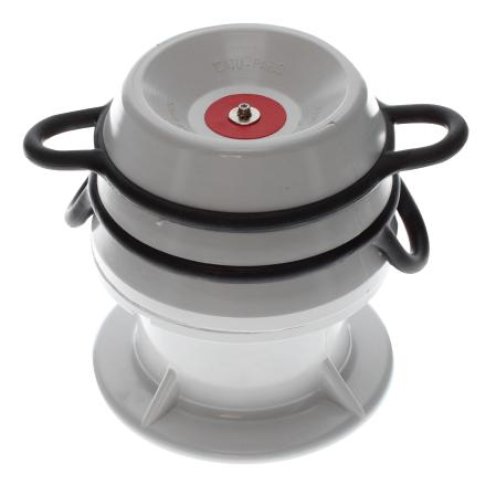
This Glove Tester is recommended by standard IEC 60903:2014 for the periodic testing of Insulating Gloves Classes 00 to 4.
