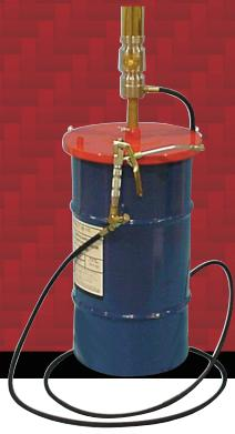
These professional delivery systems include all required equipment including a 60:1 high-pressure pump, control handle, Z-swivel, drum cover, follower plate and 8' outlet hose. Fits 35 lb., 120 lb. and 400 lb. grease containers.
