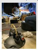
Removing and replacing fluid is now a one-person job. This Pneumatic Brake Fluid Exchanger makes brake bleeding clean and simple using compressed air and a venturi vacuum system. Use to evacuate a variety of other fluids from vehicles or small engines. Includes a bleeding tube and fluid refill bottle.
